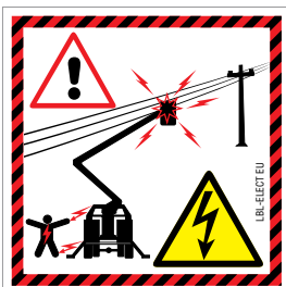
WARNING Check for overhead powerlines before use
