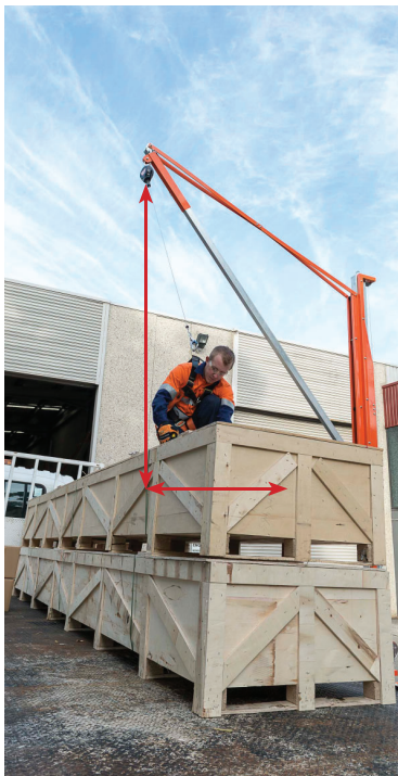
Typical Safe Working Zone for Fall Protection
