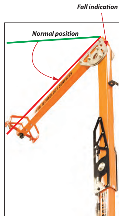
Figure 21a Overload Indication.
