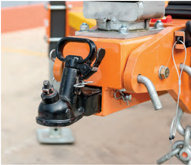
Figure 2a Standard Hitch; 50mm Ball Hitch
