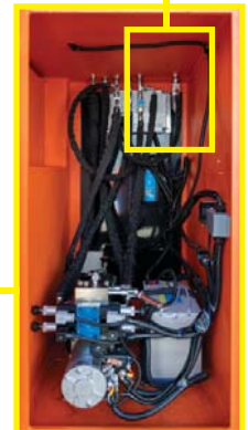
Relief valve located at the top of the hydraulic/Battery Compartment
