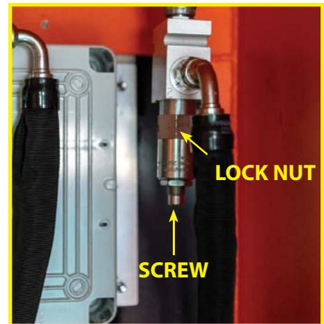
Relief valve located at the top of the hydraulic/Battery Compartment
