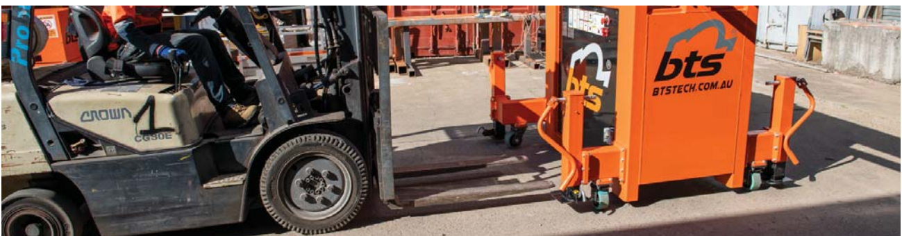
Position the fork lift only where marked (FORKLIFT POCKET)
